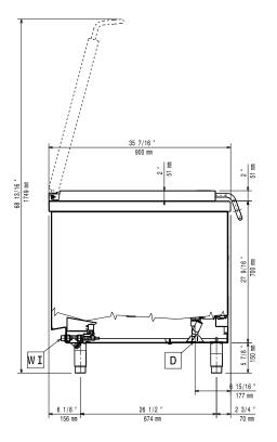
D = Drain EI = Electrical inlet (power) EQ = Equipotential screw WI = Water inlet
